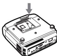
9. Tighten up the screw (a) using a Phillips screwdriver (+) to secure the lamp cover.
