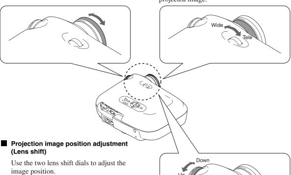
If you cannot position the projector straight in front of the screen, use the lens shift dial so that the image is centered on the screen. When you turn the lens shift dial and hear a click, the lens position is almost centred.
