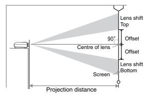
The height from the centre of the lens to the bottom of the screen will vary depending on the lens shift setting.
