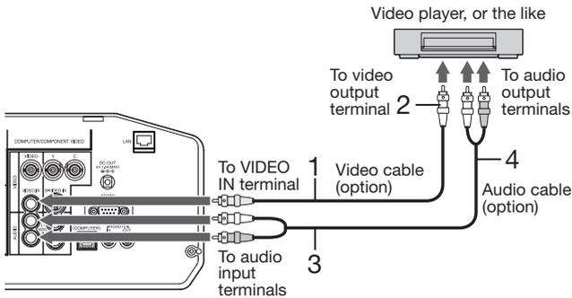
1. Connect one end of a commercially available video cable to the VIDEO IN terminal of the projector.
