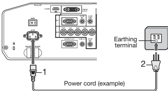
1. Plug the attached power cord into the power cord inlet of this projector.
