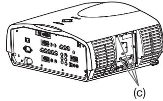
9. Tighten up the screw (a) using a Phillips screwdriver (+) to secure the lamp cover (b).
