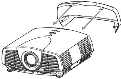
1. Fit two hooks of the terminal cover into the projector.
