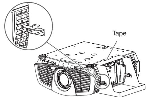
5. Detach the lamp replacement tray together with the removed lamp.
