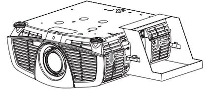
3. Secure the lamp replacement tray on the projector using the tape packed with the tray.
