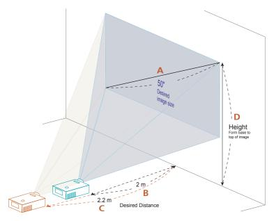
The table below shows how to achieve a desired image size by adjusting either the position or the zoom ring. Example: to obtain an image size of 50" set the projector at a distance 2 m and 2.2 m from the screen and adjust the zoom level accordingly.
