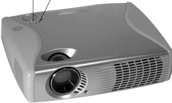
POWER Indicator STANDBY(RED) ON(GREEN)
