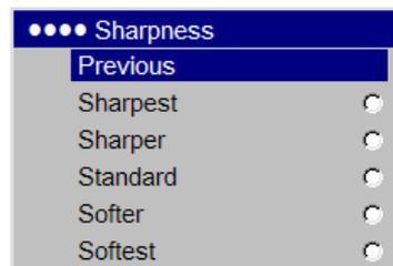
**Sharpness:** (video sources only) changes the clarity of the edges of a video image. Select a sharpness setting.
