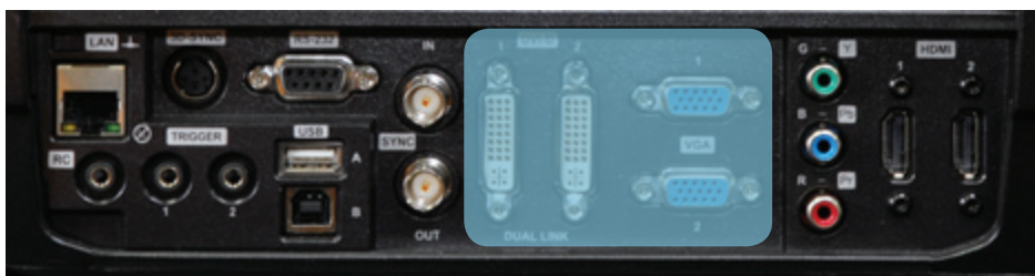
Figure 5-4. Connecting a computer source
