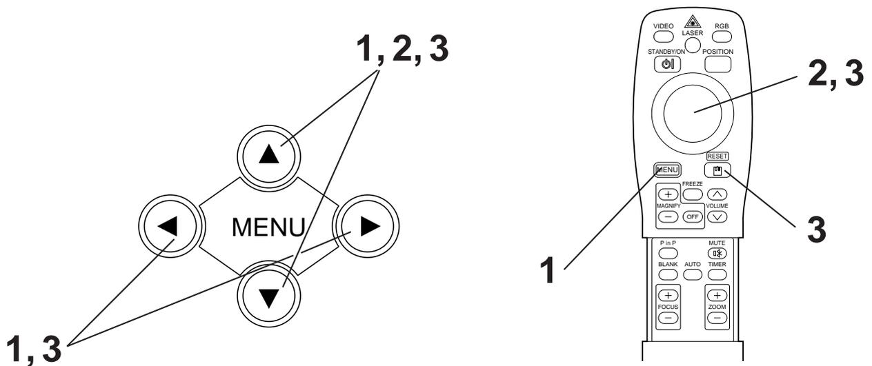
**1** Press the MENU ( ▲▼◀▶ ) buttons of the projector or the MENU button of the remote control.
