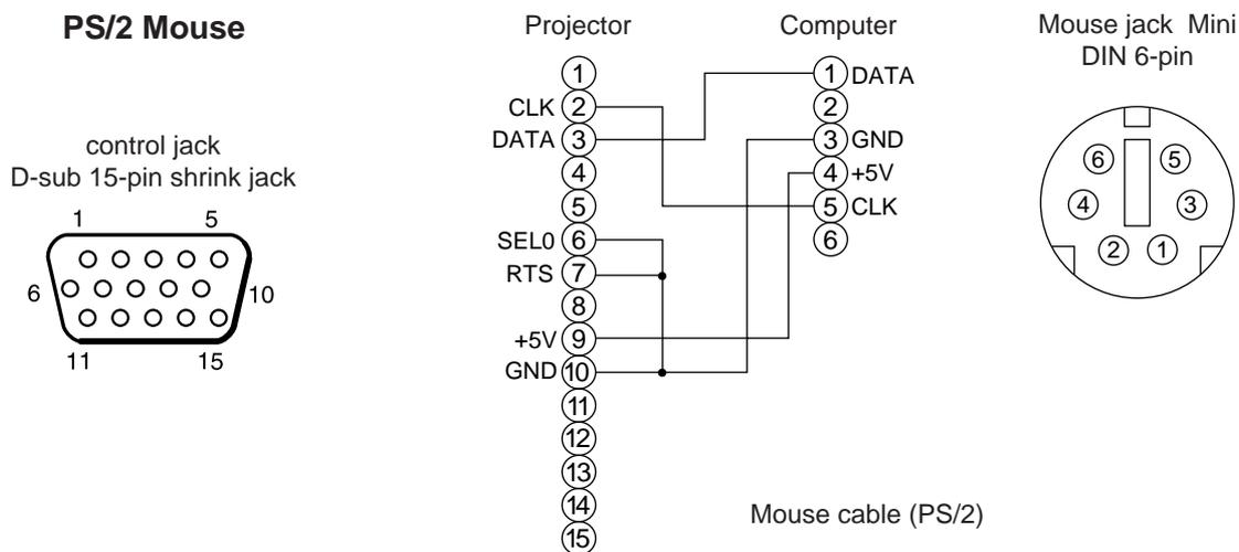
Use the mouse cable provided or a PS/2 mouse cable (for IBM and compatibles).
