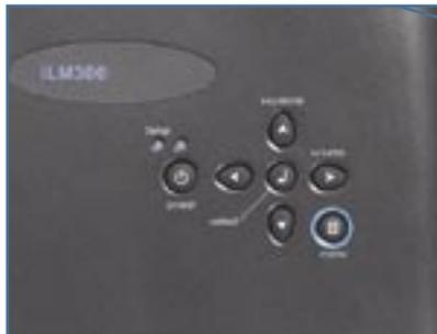
*Control panel features on the IBM iLM300 MicroPortable Data/Video Projector*
