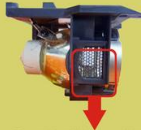
Expanded metal to prevent dangers by lamp fragment after explosion
